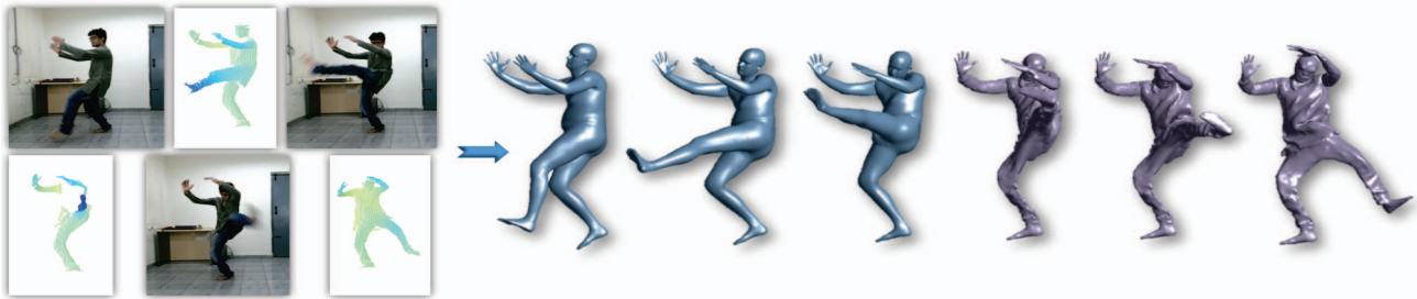
Figure 1: Left: Input to our system (only depth maps are used), Right: Output of our system, where first three meshes show SMPL model tracked over time and last three meshes show Consensus meshes , reposed using SMPL
