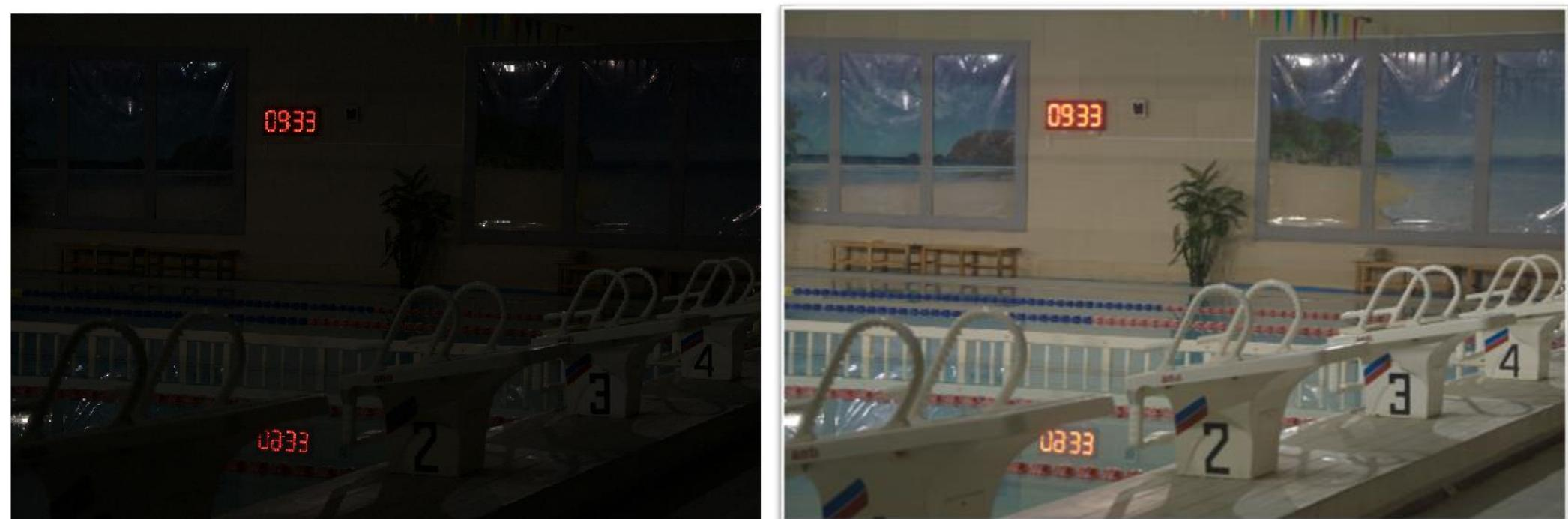
**Simulated Exposure Fusion (SEF):** Render virtual *exposure stack* from the single image → global enhancement → merge using Exposure Fusion (EF) algorithms.
